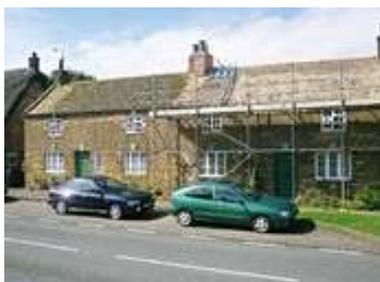
4.23 Cement and sand mortars shouldn't usually be used on roofs, as it will not allow any expansion of the roof covering and may crack and fall off. However during the survey of the village in August 2008 one property with an original Colleyweston slate roof (referred within this region as Colly roofs) was noted as then being 'repaired' with pointing on its roof. English Heritage (EH, Northampton Office)
